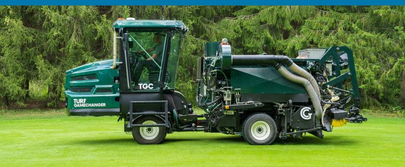
The entire hydraulic system of the work machine has been designed and tested by Comatec. The hydraulic system consists of a power and pump unit, hydrostatic drive, steering, and the various different hydraulic actuator circuits.
